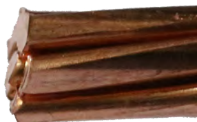
Cut made with special M&P scissors.
